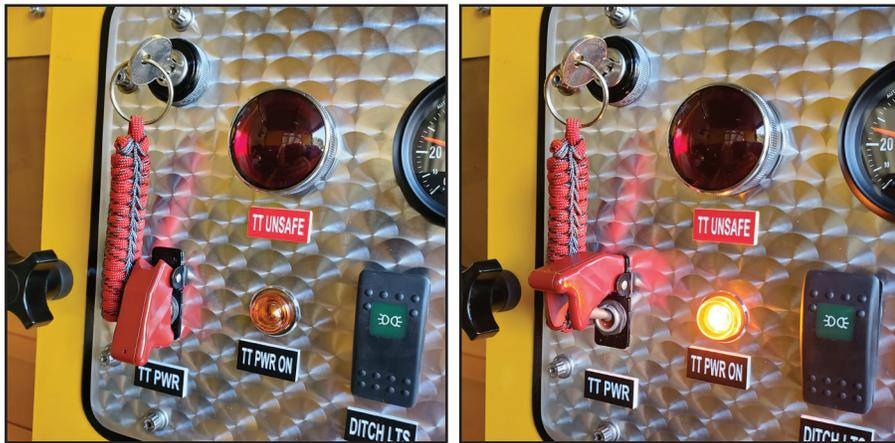
The “turntable unsafe” warning is also a standalone system. It is powered by the ignition side of the starter switch, so anytime the ignition switch is ON, the warning system is powered regardless of any other switch position on the motorcar. Ignition “on”-- turntable warning “on” works for me. The
